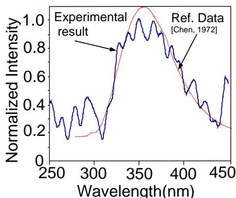
Fig. 8: The net output from the tryptophan sample, obtained by subtracting the curve of Fig. 7 from that of Fig. 6. The reference emission curve of tryptophan [6] has been superimposed.
