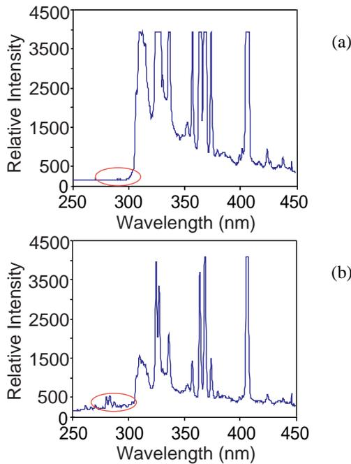
Fig. 5: (a) Light transmitted through tryptophan shows that the peaks near 280 nm have been absorbed; (b) These wavelengths are transmitted through the control sample of water.
