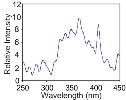
Fig. 6: Optical emission measured along optical path II (as shown in Fig. 2) indicating the existence of the direct fluorescence of tryptophan by the broad peak between 325 nm and 425 nm.
