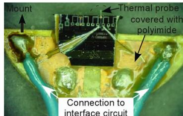
Fig. 3: A mounted scanning thermal probe with the base covered with a polyimide (PI2613<sup>TM</sup>) layer for working in aqueous environments.
