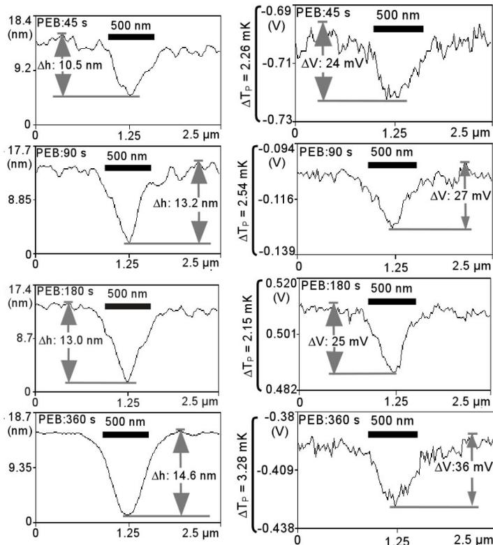
Fig. 9: Topographic (left) and thermal (right) line scans of a latent image in UV6<sup>TM</sup> with varying PEB time at 130°C.
