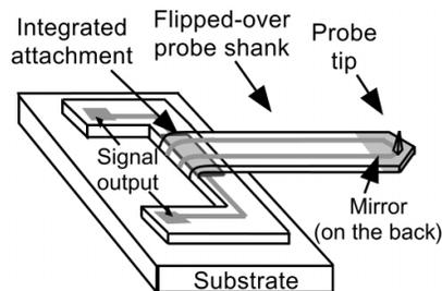
Fig. 1: Schematic of the ultracompliant polyimide thermal probe.
