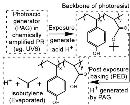
Fig. 8: In UV6<sup>TM</sup>, PAG acid deprotects the backbone during PEB for subsequent dissolution in the developer
