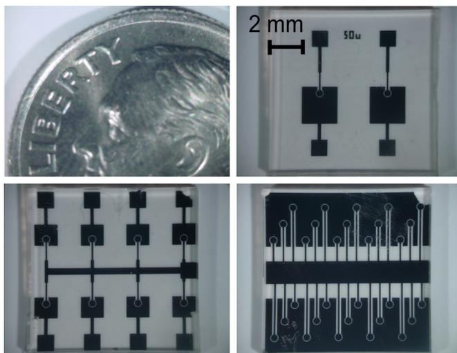
**Fig 2:** (a-top left): A US dime. (b-top right): Two junction chip. (c-bottom left): Single anode with eight cathode chip. (d-bottom right): Single anode with two cathodes each having fifteen junctions chip.
