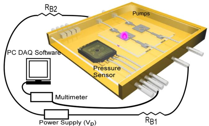
Fig. 1: Schematic of a cavity, pressure sensors, electrode configuration, power, and readout circuitry.  $R_{B1}$  and  $R_{B2}$  are 1.2 M $\Omega$  ballast resistors which limit the current flowing through the arc between electrodes. All electrode pairs have a 50  $\mu$ m discharge gap.
