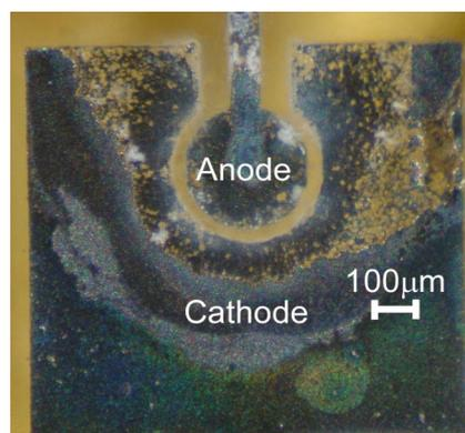
Fig. 6: Remains of the top electrode of the second pump design, illustrating areas of complete titanium sputtering.
