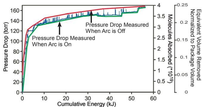
Fig. 5: The pressure drop as a function of the cumulative energy supplied to the discharge. The upper and lower trend lines respectively show the pressure reading when the discharge is interrupted (causing spikes as the pressure stabilizes without an increase in energy) and when the discharge remains on. The corresponding number of gas molecules removed at room temperature, and the fraction of the cavity volume evacuated, are also noted on the right-hand-side Y-axes.
