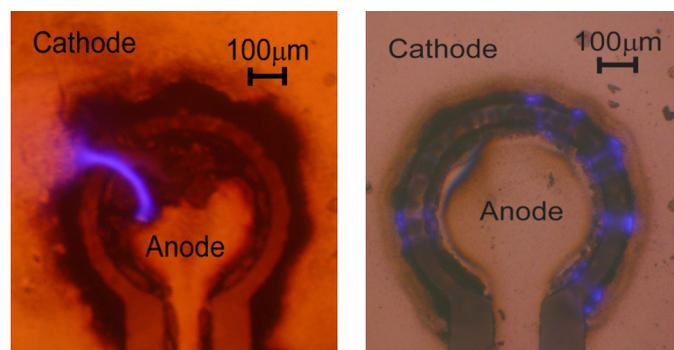
Fig. 7: (a-left) Hybrid discharge and sputtered electrodes. Hybrid discharges such as this occurred when the arcing current was limited to 50  $\mu$ A. (b-right) Multiple discharges created by high current. Discharges such as this sputtered a majority of the titanium.
