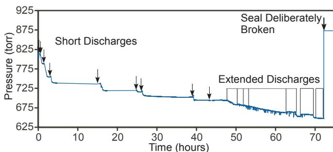
Fig. 4: Pressure drop in the cavity over time. Fifteen consecutive discharges dropped the pressure 168 Torr. The pressure remained stable over periods of ten hours of pump inactivity and returned to room pressure when opened.
