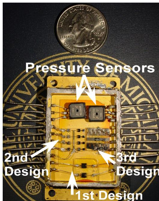
**Fig. 3:** Package after opening with two pressure sensors and all three pump designs included.
