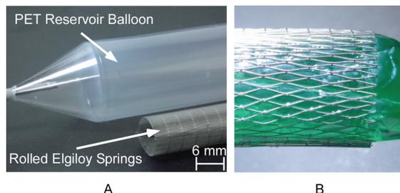
Figure 5: A) Components used in an 18.8 mL reservoir. B) Filled balloon reservoir in an expanded sleeve.
