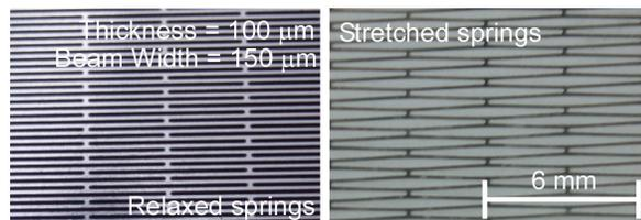
Figure 3: Left: Relaxed Elgiloy® spring mesh. Right: Stretched springs. Cell windows are each 600  $\mu\text{m}$  x 6 mm
