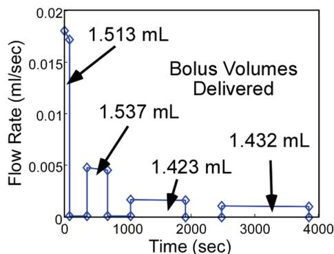
Figure 10: Programmed delivery of 6 mL in four boluses of 1.5 mL. This demonstrates the ability to regulate volume using the pressure sensor. The volume delivered was 5.971 mL.
