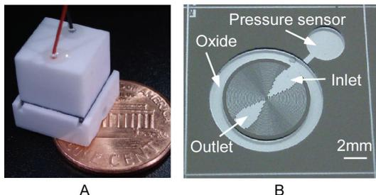
Figure 2: A) A valve with a Macor header B) The top of the valve. The pressure sensor cavity is clearly shown.
