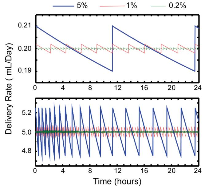
Figure 8: Calculated change in flow rate over time due to changes in valve constriction at various error rates. The frequency of valve adjustments decreases over time due to non-linearity in the reservoir.
