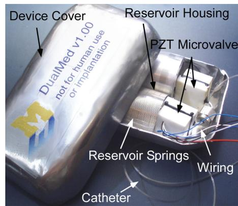
Figure 6: The prototype contains two reservoirs in a casing to prevent them from interfering with each other, and allows two medications to be regulated independently. This preliminary prototype is not refillable via injection ports.
