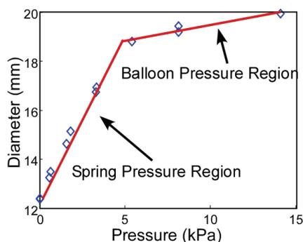
Figure 9: Reservoir pressure generated for various balloon/sleeve distension. From 12 mm to 19 mm, the pressure is generated by the springs. Beyond 19 mm, the balloon elasticity changes the profile. Fully inflated, the reservoir is 20 mm in diameter and generates almost 15 kPa.
