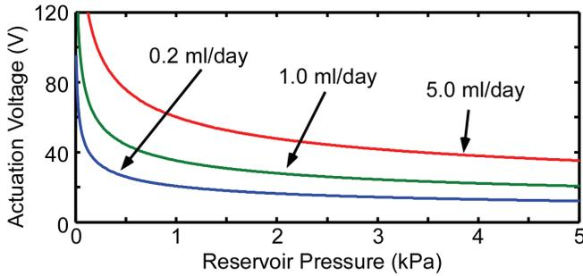
Figure 7: Calculated voltage needed to actuate the valve to maintain a set flow rate for various reservoir pressures
