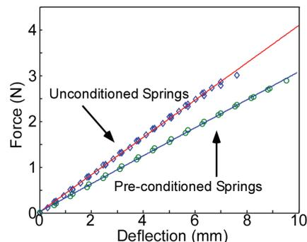
Figure 4: Load characteristics of the mesh springs as a function of linear conditioning (stretching). The unconditioned spring constant is 407.3 N/m and the pre-conditioned spring constant is 305.7 N/m.
