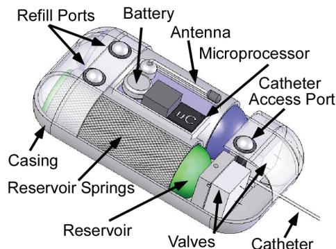
Figure 1: Two reservoirs are pressurized with compressive sleeves and regulated by independent microvalves to control delivery rates. The device is implanted into the abdominal region, and the catheter is subcutaneously routed around the side of the body, up the back, and implanted into the center of the spinal column.
