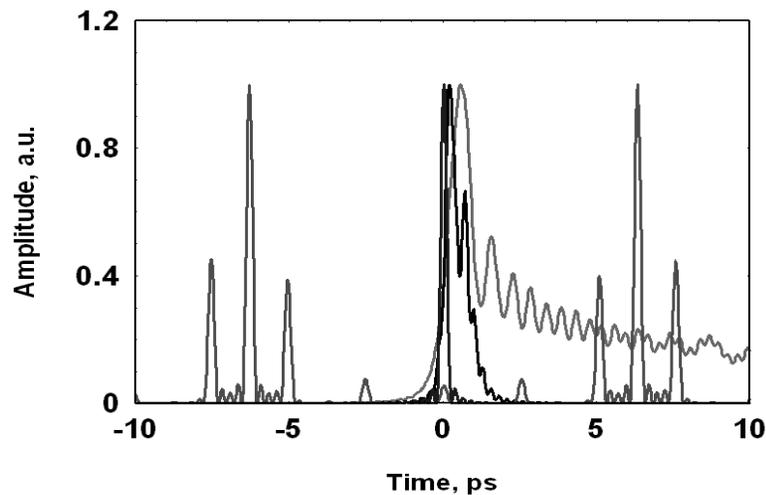
Fig. 5. Numerically simulated traces of the FBG-MEMS shaped pulses. Blue – bandwidth limited pulse, red – periodic phase modulation, black and purple – various amount of induced cubic phase.
