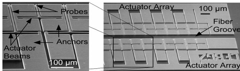
Figure 2: A scanning electron microscopy (SEM) image of the micro-fabricated actuator array and a fiber groove for 80- $\mu$ m. Actuators are lined up on both sides of the fiber groove. Each actuator consists of a floated V-shaped bent-beam and a floated probe attaches to the bent-beam at the apex.
