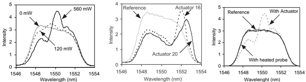
Figure 4: On the left, the spectral change of an actuator was driven at different power level is shown. In the center, two spectral changes generated by different actuator both driven at 500mW are shown. On the right, the electro-thermal actuator induced spectral change is compared to the spectral change caused by a direct heat-up of the grating using a 350 °C probe. The direct heat-up spectral change is relatively small compare to the actuator induced spectral change.
