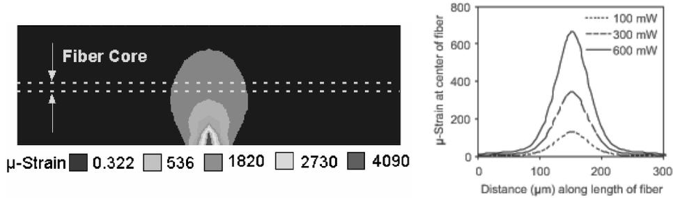
Figure 3: FEA showing strain penetration transversely and along the fiber core. In a fiber core a strain of up to hundreds of micro-strain can be created. The inter-actuator cross-talk is not significant as shown in the right plot.
