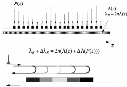
Figure 1: CFBG maps different frequency components to different effective-reflection-position where the Bragg condition is locally satisfied. By applying localized pressure, the local Bragg-wavelength and, therefore, the phase relation between different frequency components can be controlled.
