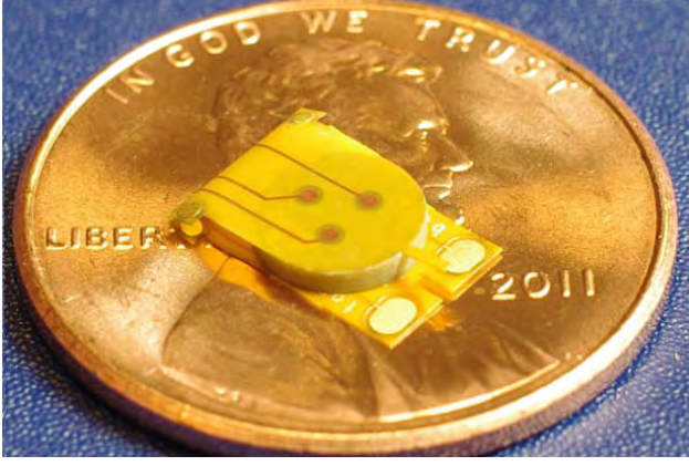
Fig. 3. The high voltage generator against a U.S. cent.
