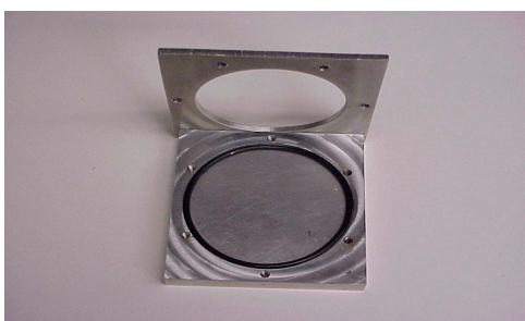
Fig. 2. Fixture used for casting polyNIPAAm films.
