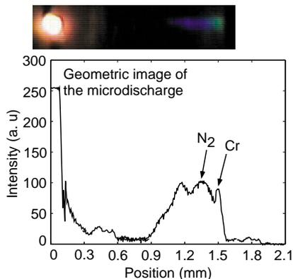
**Fig. 7:** Measured diffraction pattern obtained from a Cr contaminated water sample using the planar structure with optical sys. A.
