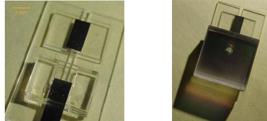
Fig. 5: Optical micrographs of a partially assembled (a-left) and finished planar device (b-right). Chip area is ~ 9 mm X 15 mm.
