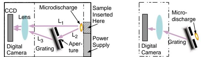
Fig. 3: (a-left): *Optical system A*, designed to include the geometric image of the microdischarge (not to scale). System only requires external camera and power supply for operation. (b-right): *Optical system B*, designed to exclude the geometric image.
