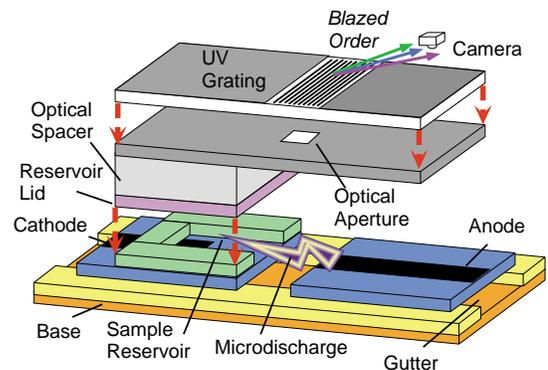
**Fig. 1a:** Exploded view of the “planar” device. The thick arrows indicate how the system is assembled
