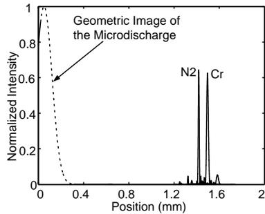
Fig. 4: Calculated spectrum from Cr contaminated water with the geometric image of the microdischarge (dashed line). Configuration in Fig. 3a excludes geometrical image.
