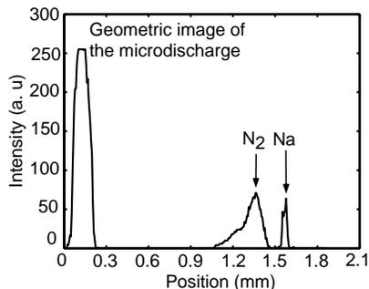
**Fig. 10:** Measured diffraction pattern obtained with capillary tube plasma using Na contaminated water.
