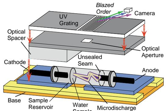
**Fig. 1b:** Schematic of the “capillary tube” device. The structure is held vertically during operation
