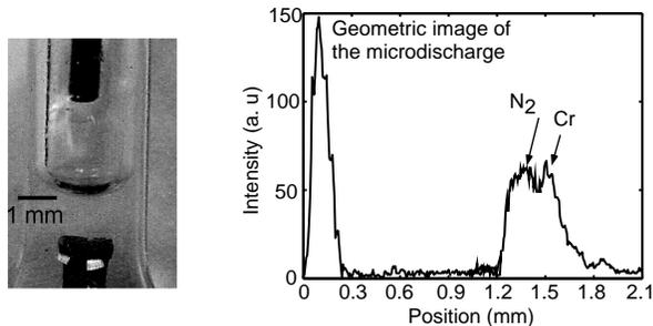
**Fig. 9:** (a-left): Close-up of capillary tube with diffraction grating removed, showing microdischarge; (b-right): Measured diffraction pattern obtained with capillary tube plasma using Cr contaminated water (optical sys. A).
