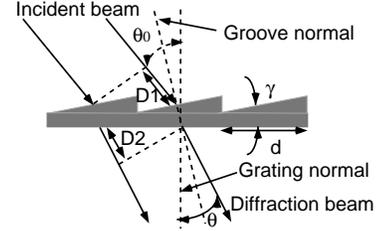
Fig. 2: Illustration of a transmission blazed grating.
