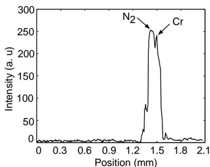
**Fig. 8:** Measured diffraction pattern from planar structure using Cr contaminated water sample (optical sys. B).
