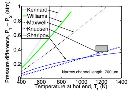
Fig. 7: Total pressure drop for the narrow channel as function of T<sub>1</sub>. The box shows experimental data.
