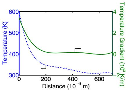
Fig. 5: The local temperature and its gradient along the channel for a single stage pump (ANSYS).
