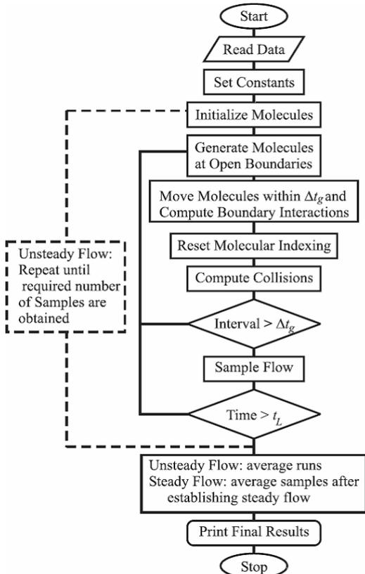
Fig. 2: The computational flow for DSMC technique
