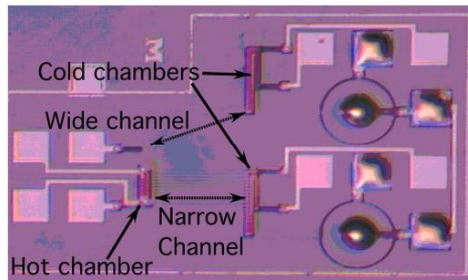
Fig. 4: Photograph of a single stage Knudsen pump used for experimental verification [8]
