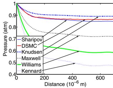
Fig. 6: Pressure distribution along the channel, as predicted by various models using temperature profile from Fig. 5.
