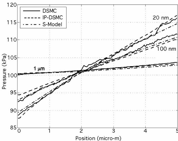
Fig. 8: Pressure profiles for various channel heights, corresponding to a test case for which the temperature profile was assumed to be linear and ΔT = 300K. The results from DSMC, IP-DSMC and from the S-model are in close agreement with each other for all three cases.
