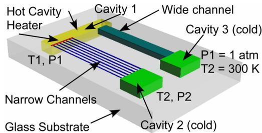
Fig. 3: Schematic layout of a single stage Knudsen pump.
