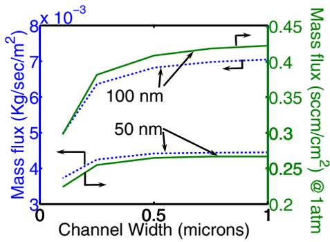
Fig. 11: Mass flux and equivalent flow at ambient pressure for 50 nm and 100 nm channel heights.
