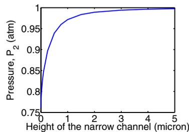
Fig. 9: With P<sub>1</sub> at atm., reducing channel height can lead to significantly improved pressure ratios. Width of channel assumed at 10 μm.
