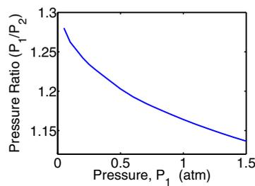
Fig. 10: Pressure ratio (P<sub>1</sub>/P<sub>2</sub>) improves for lower hot end pressures (P<sub>1</sub>). (Assumes channel height = 0.1 μm and channel width = 10 μm.)
