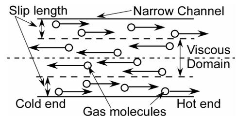
Fig. 1: Thermal Transpiration at molecular level.
