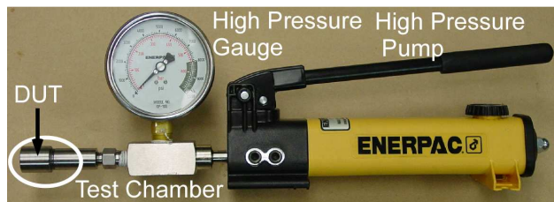
Figure 5: Test set-up used to apply high pressure oil to the sensor.
