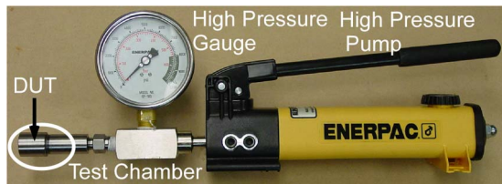
Fig. 11. Test setup used to apply high-pressure oil to the sensors.
