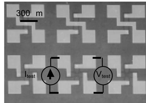
Fig. 7: SEM of six test structures used to measure contact resistance between the various layers. The circuit illustrates the proper connection for a 4-wire resistance measurement.
