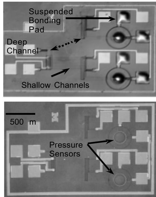
Fig. 3: Photograph (upper) and SEM (lower) of a vacuum encapsulated test structure containing pressure sensors, shallow and deep channels, top and buried metal layers, suspended polysilicon heaters, and lead transfer from the top metal to the polysilicon layer and to the buried metal layer.
