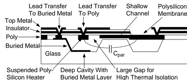
Fig. 1: Cross-section showing some of the features that the presented process provides.
