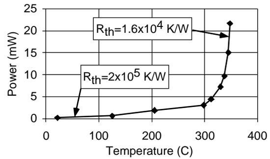
Fig. 10: Power required to heat a 1mm long suspended polysilicon heater to a given temperature, assuming that the TCR measurement of Fig. 9 is valid over the entire range.
