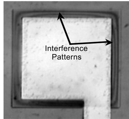
Fig. 6: Photograph of a suspended bonding pad. Interference lines can be seen between the metal and the bonding polysilicon due to the deflection of the pad due to atmospheric pressure.
