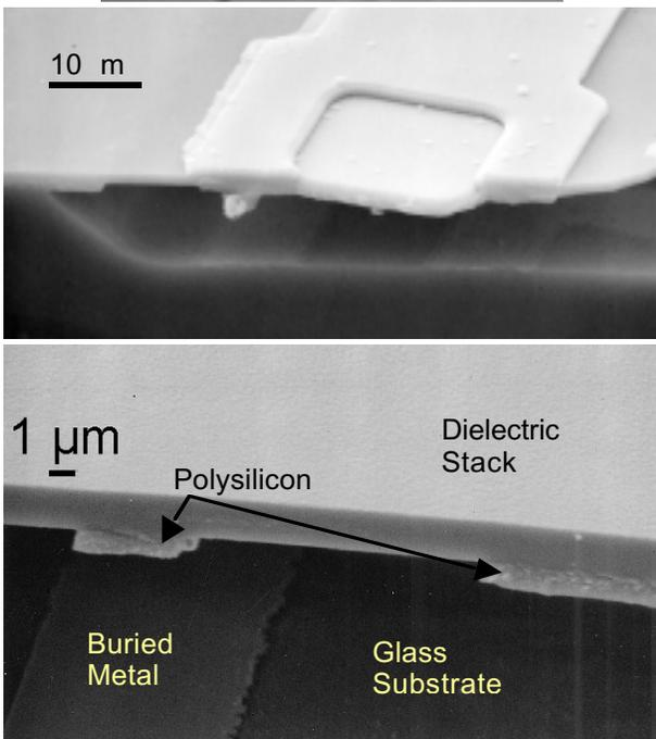
Fig. 5: (a-upper) Optical micrograph of a lead transfer; (b-center) SEM of a suspended lead-transfer from the top metal to a polysilicon layer. (c-lower) SEM of a deep channel showing the buried metal and suspended polysilicon layers.
