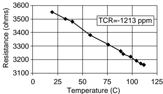
Fig. 9: Plot of resistance versus temperature of a polysilicon heater. The TCR is  $-1213$  ppm.
