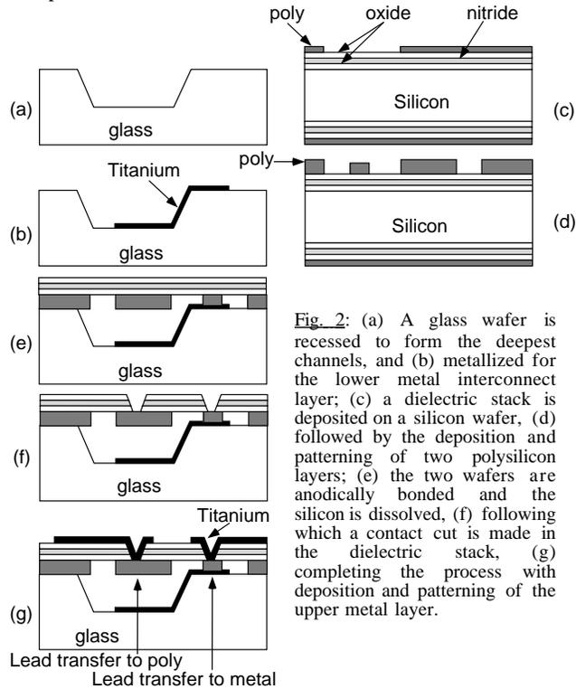
Fig. 2: (a) A glass wafer is recessed to form the deepest channels, and (b) metallized for the lower metal interconnect layer; (c) a dielectric stack is deposited on a silicon wafer, (d) followed by the deposition and patterning of two polysilicon layers; (e) the two wafers are anodically bonded and the silicon is dissolved, (f) following which a contact cut is made in the dielectric stack, (g) completing the process with deposition and patterning of the upper metal layer.
