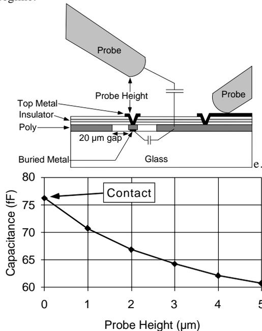
Fig. 8: (a-upper) Parasitic capacitance test set-up. (b-lower) Measured capacitance between a test probe and the bonding polysilicon as a function of the probe height above a lead-transfer structure.
