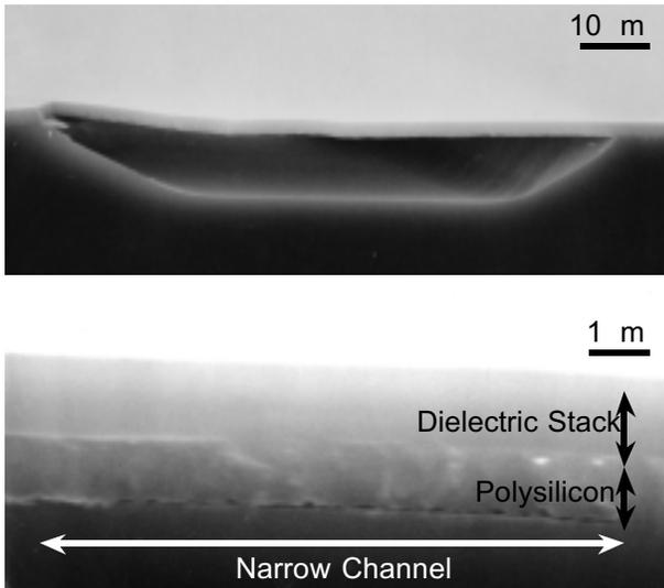
Fig. 4: An SEM of a deep channel (upper) and shallow channel (lower). The height of the shallow channel is only 100 nm, two orders of magnitude smaller than the height of the deep channel.
