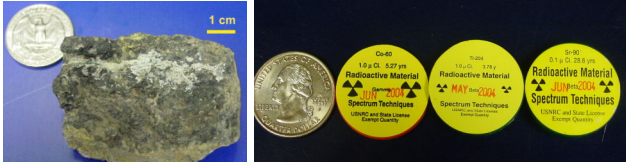
Fig. 7: Naturally occurring uranium ore (left) and calibrated 0.1-1 \mu Curie isotope samples of various materials used to test devices.
