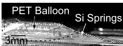
Fig. 7: Actuated silicon torsion springs with a PET angioplasty balloon acting as a liquid reservoir.
